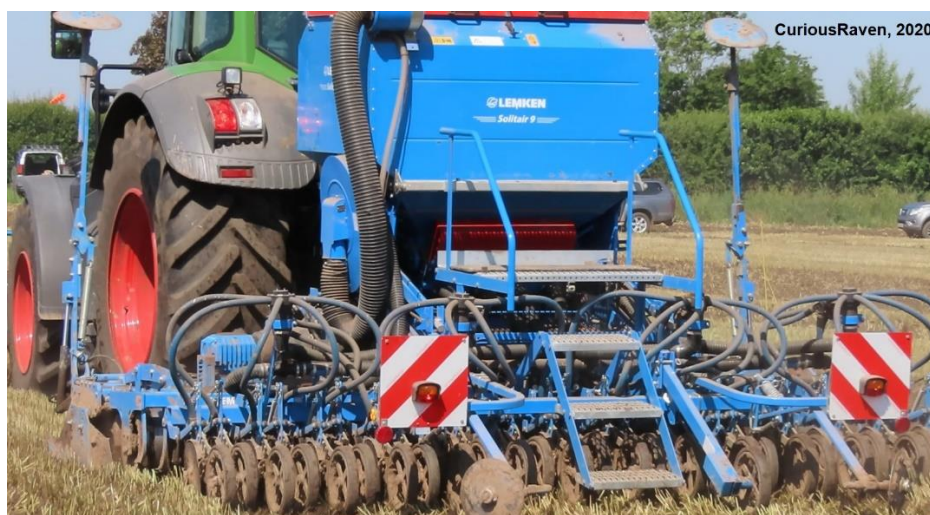
Figure 4. Planting equipment at Caynton, Lilyhurst and Tibberton. Lemken Solitair 9.
